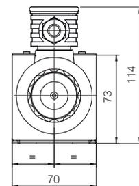
Note: for option /B the solenoid is at side of port A (only for DHZE-A-05 and DKZE-A-15)
