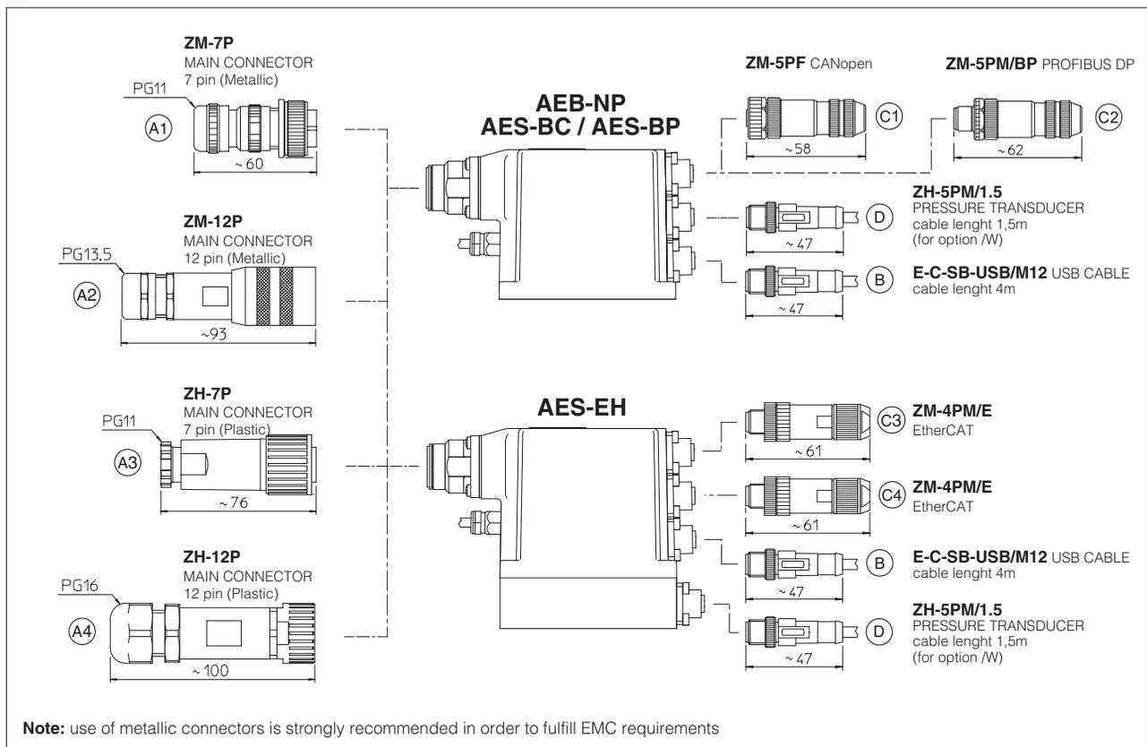
14 MODEL CODES OF MAIN CONNECTORS AND COMMUNICATION CONNECTORS - to be ordered separately
