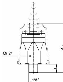
N.A. = The pressure switch closes an electric contact when it reaches the fixed pressure
